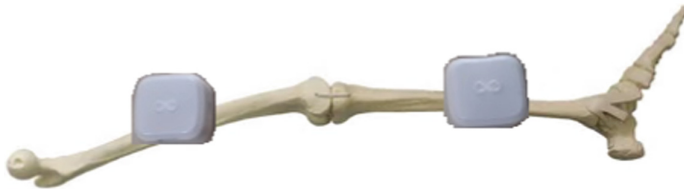
Fig. 3. A sawbone leg model with Muse V3 sensors placed on it.
