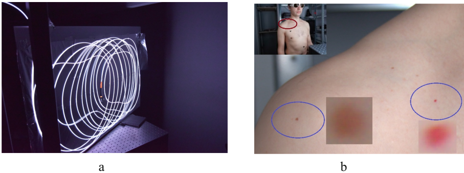
Fig. 1. The planar RGB illuminator - tangled side-emitting optical fiber (a) and an example of high-resolution skin color image obtained under such illumination (b).
