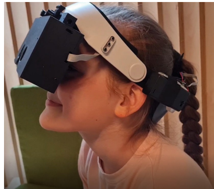
Fig. 1. The head-mounted module of the upgraded vision screening and training prototype.
