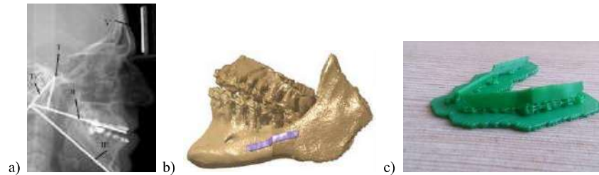
Fig 2 a) X-ray scan with basic geometry b) Solid model of the personalized plate created over scanned data by using MAF c) printed models of the plate implants (left and right) [8, 11]
